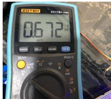
**Gambar 10.** Pengukuran Kaki Basis Ke Emitor
