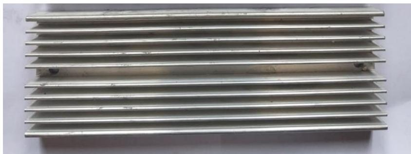
Gambar 11. Heatsink sirip 10.
