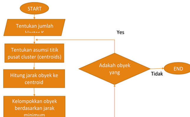
Gambar 4. Algoritma Flowchart Clustering K-Means
