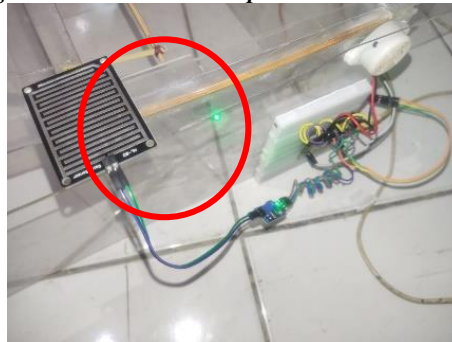
Gambar 7. Implementasi Rangkaian Sensor Raindrop
