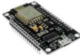
**Gambar 2.** NodeMCU Esp8266
