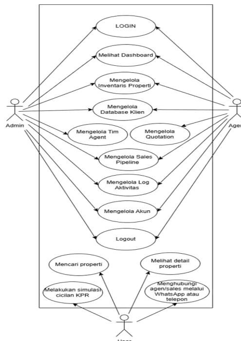
Gambar 2. Use Case Diagram Sistem CRM
