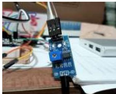
**Gambar 10.** Modul Sensor Api
